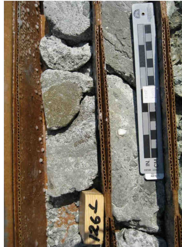
Sheared interval strong quartz-sericite-pyrite alteration
