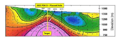
Chargeability Section: Old Hole SH10 stopped just short of anomaly, ended in altered intrusive with quartz veinlets and disseminated sulphides.
