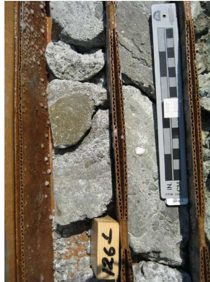
Sheared interval strong quartz-sericite-pyrite alteration
