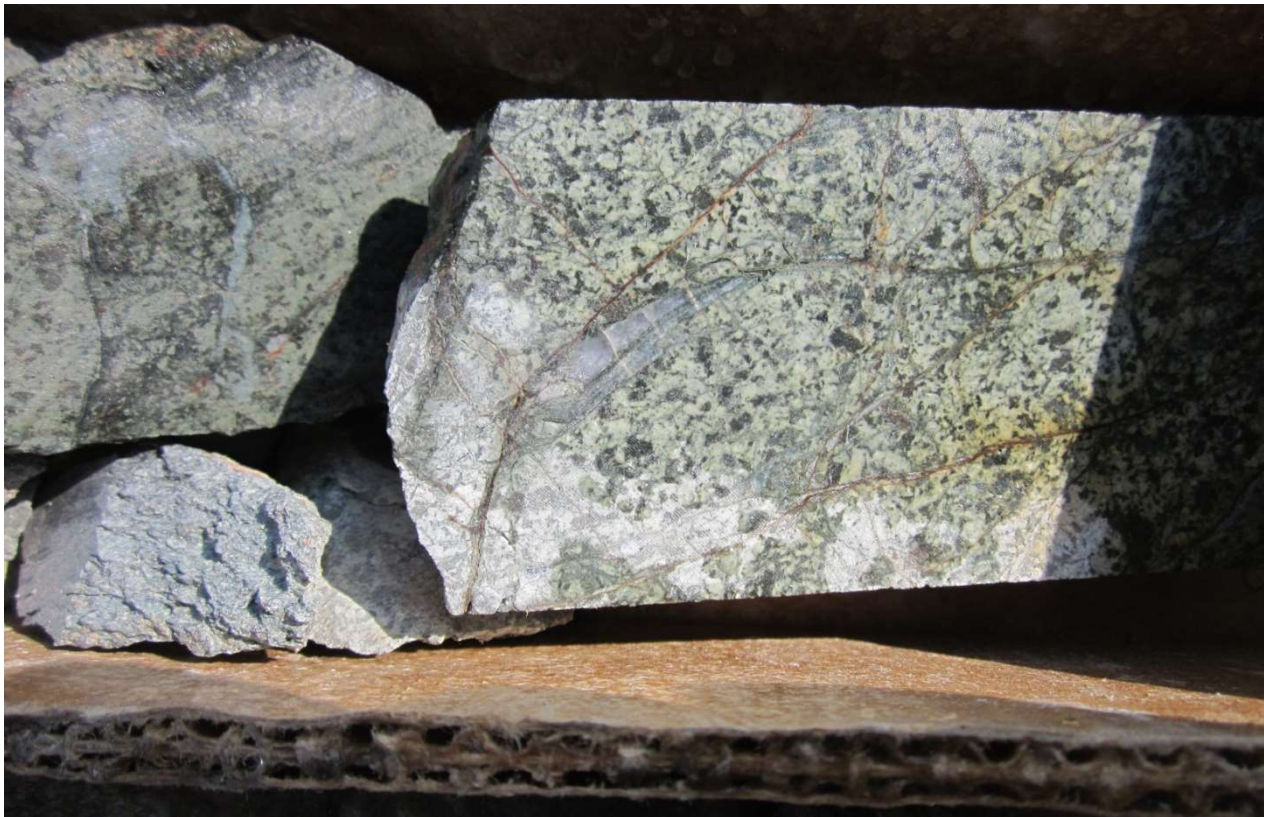
Figure 10.5 Albitized Diorite Porphyry in Hole SHK97-2
