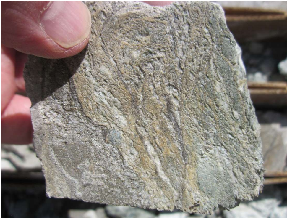
Figure 10.7 Sheared Pyrite-Illite Altered Rock at ~45m in Hole 11C-1
