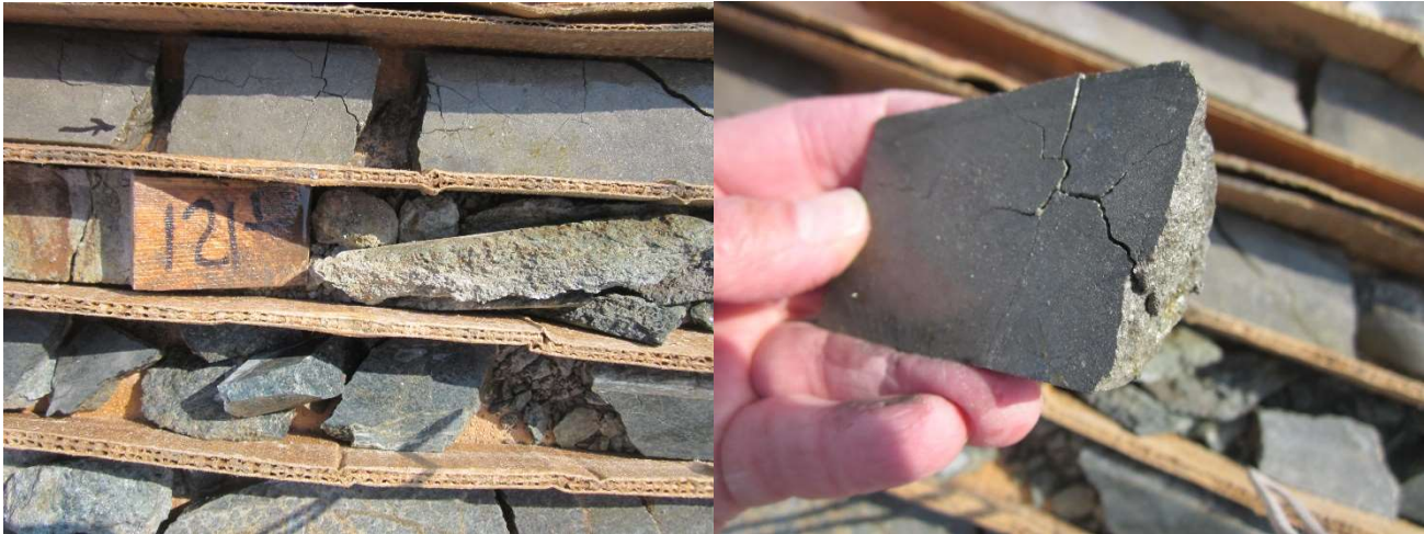
Figure 10.4 Copper-Gold Bearing Pyrite Vein at 36.6m in Hole SHK97-2
