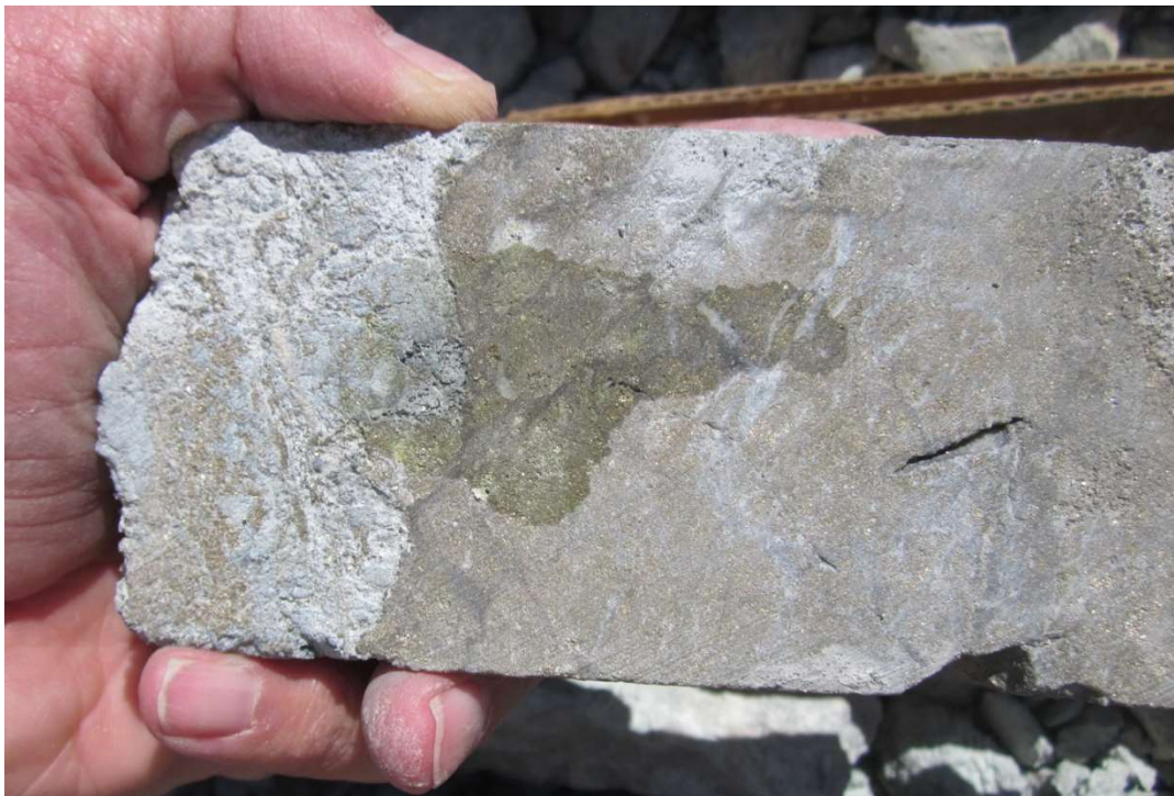
Figure 10.6 Copper-Gold Bearing Pyrite Vein at ~44.5m in Hole 11C-1
