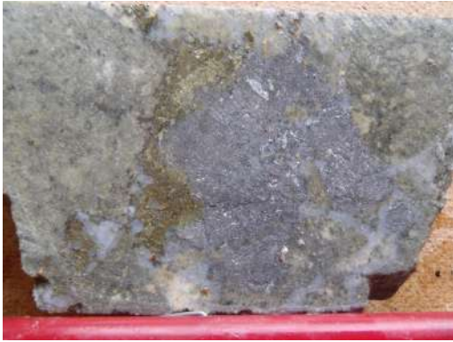
Hole GZBX11-003 (at 147 m) aspy clot ringed by py-cpy: interval grades 5.94 g/t Au, 19.7 g/t Ag, 0.18% Cu
