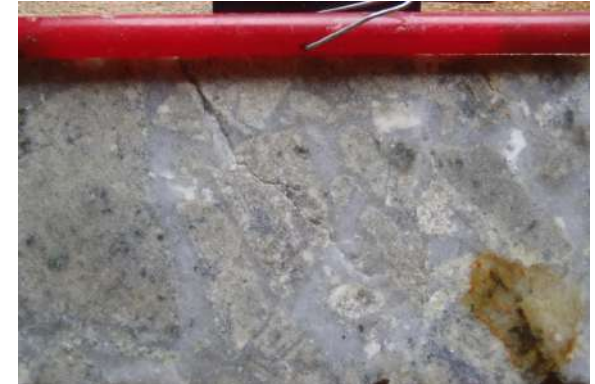
Breccia formed by invasion of silica-ankerite veins.
