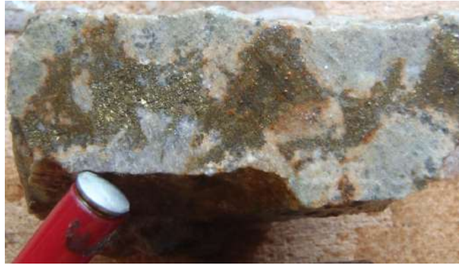
Patchy py-cpy in fractures with aspy disseminated and in clumps: interval grades 7.48 g/t Au, 34.5 g/t Ag, 0.16% Cu
